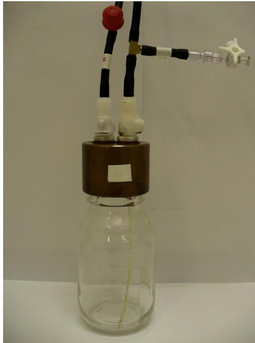
**Fig. 1.** Fermentation unit. The T-tube was used for liquid sampling (volatile fatty acids determination); the red rubber suba seal was used for gas sampling with a gas tight syringe. (For interpretation of the references to colour in this figure legend, the reader is referred to the web version of the article.)
