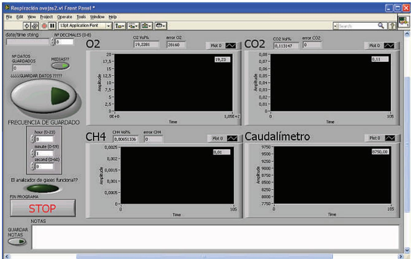
Fig. 3. Panel of the LabVIEW program for monitoring gas analyser and the flow meter.
