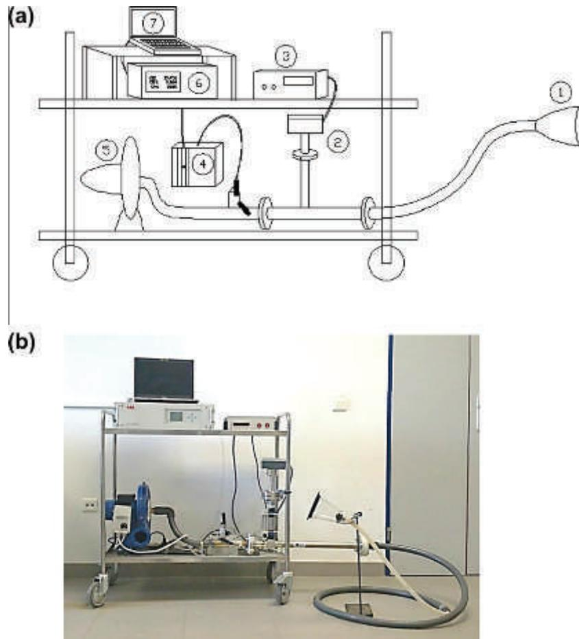
**Fig. 2.** Diagrammatic representation of the respiration mask device. (a) 1 – mask; 2 – thermal mass flow meter; 3 – transducer and totaliser; 4 – pump and flow meter; 5 – fan; 6 – gas analyser; 7 – laptop with software included. (b) Picture of the system.
