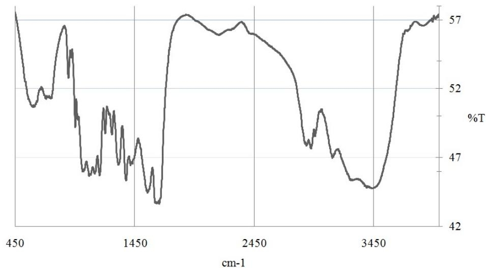
**Figure 2.** FTIR spectra of chitin fermented BSF larvae using *Bacillus subtilis* (T4).
